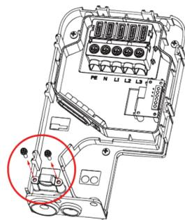
2. Strip the individual wires by about 7 to 10 mm (0.3 to 0.4in). Wrap the terminal blocks in the accessory kit to the core. Use pliers to crimp the terminals firmly.
